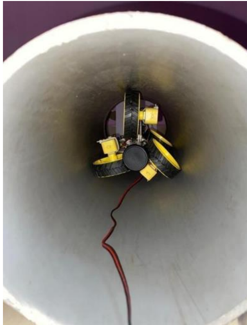
Fig 5.9.1 : After insert the bot in pipeline.
