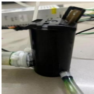
Fig 4.6: 12v dc water pump
