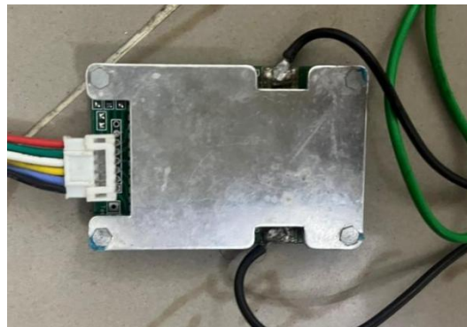
Fig 4.7: Battery Management System
