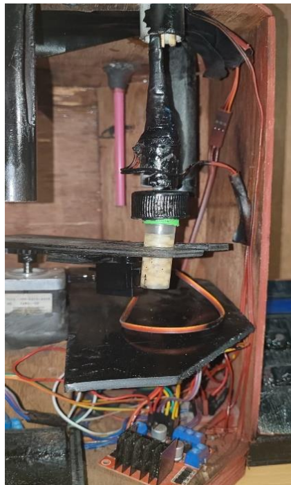
Fig:5.3: Capping is done at the capping station.
