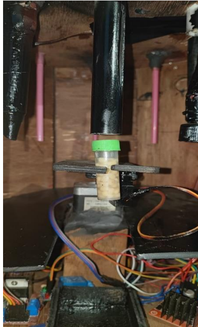
Fig:5.4: Dropping of the bottle at the dropping station
