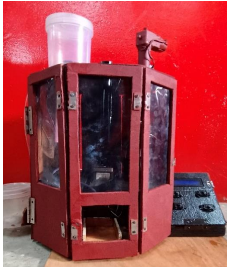
Fig:4.17: Automatic Homeopathy Pills Filling and Capping Machine
