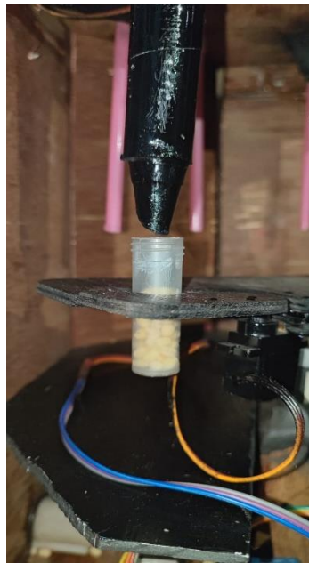
Fig:5.1: Pills filled in the pills filling station.
