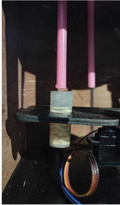
Fig:5.2: Drug dilution is filled at the drug dilution filling station.
