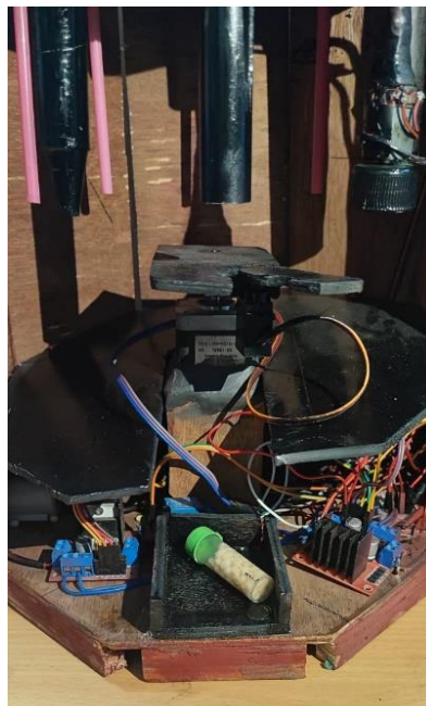
Fig:5.5: Homeopathy pills and drug filled bottle dropped into the tray.
