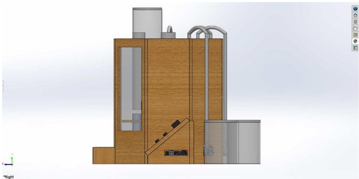
Fig:4.15: Right view of Automatic Homeopathy Pills Filling and Capping Machine.
