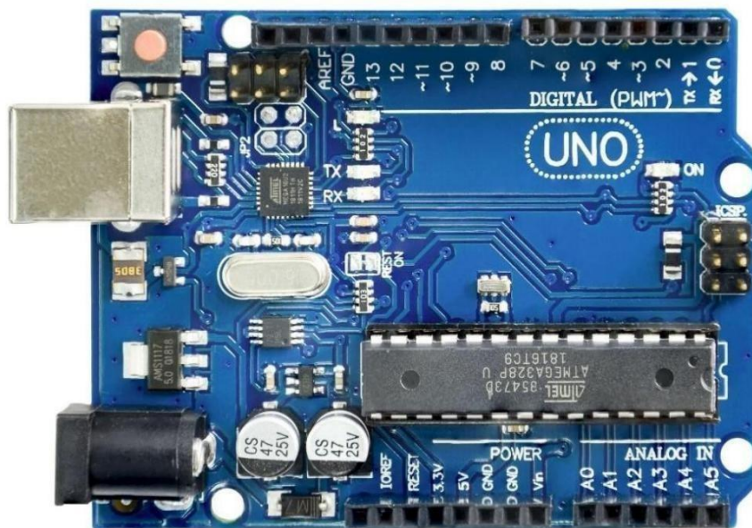
Figure 4.10: Arduino Uno R3
