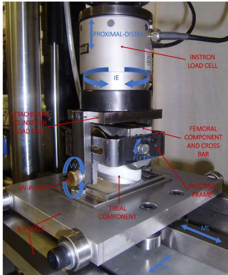
Fig: 4.3 Rotational stability testing rig.
