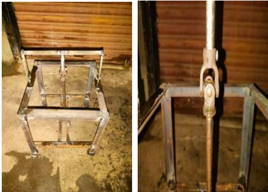
Fig:5.20 Fabrication of Knee stimulator
