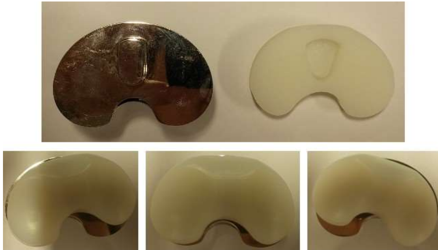
Fig: 4.7 The mobile bearing version of the Saiph Knee. Top left: the polished tibial tray with post. Top right: the backside of the UHMWPE tibial bearing with the rotation slot visible in its centre. Bottom: a right-sided bearing in place on top of the symmetrical tibial tray at the internal (left), neutral (centre) and external (right) limits of its rotation.
