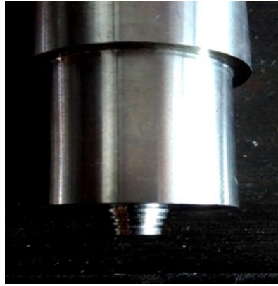
Fig:4.3 : FSW tool with threaded Pin
