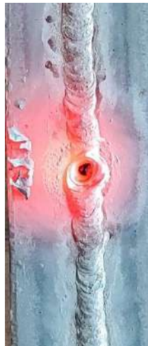
Fig: 3.1: Deformed weld metal while welding.
