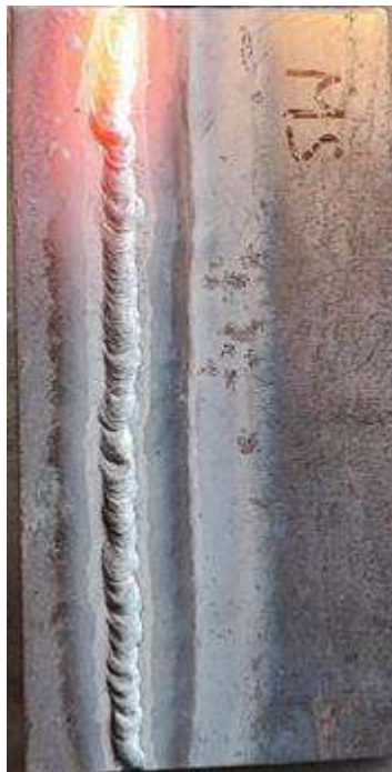
Fig:5.5 : Mild steel welded under the weld rig
