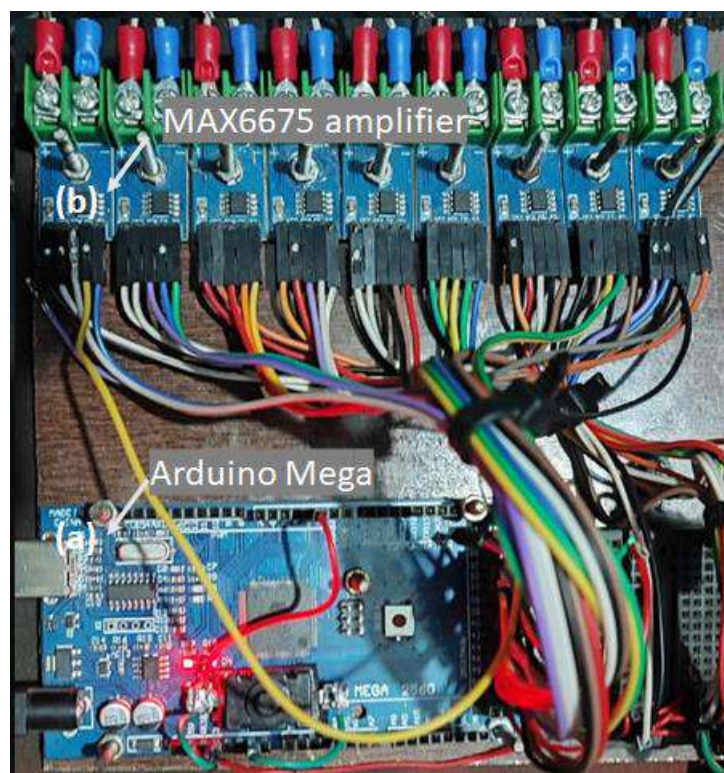
Fig:4.4 : Circuit diagram for interfacing Arduino with amplifier
