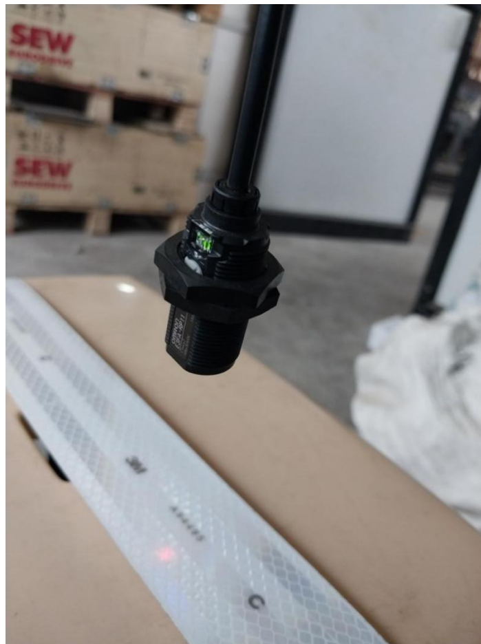
Fig 4.9 Senses reflective signals from tape
