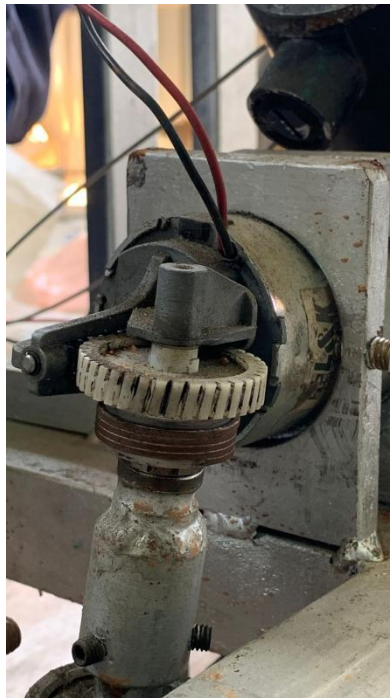
Fig 4.6 Wiper motor in steering System
