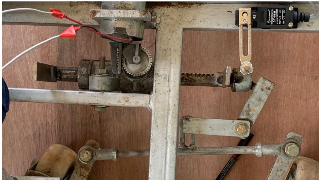
Fig 4.4 Free Wheels with Ackermann steering
