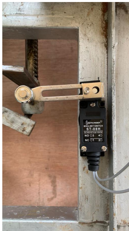
Fig 4.5 Limiter Switch in steering control
