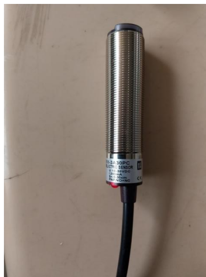
Fig 4.10 Photo electric sensor (Diffuse Reflective Sensor)
