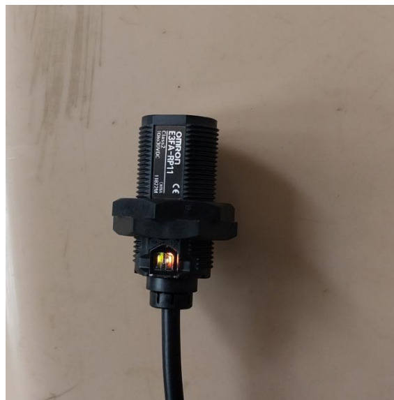
Fig 4.7 Omron Retro Reflective Sensor
