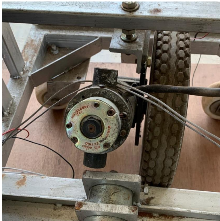
Fig 4.3 DC Motor - Driven Motor
