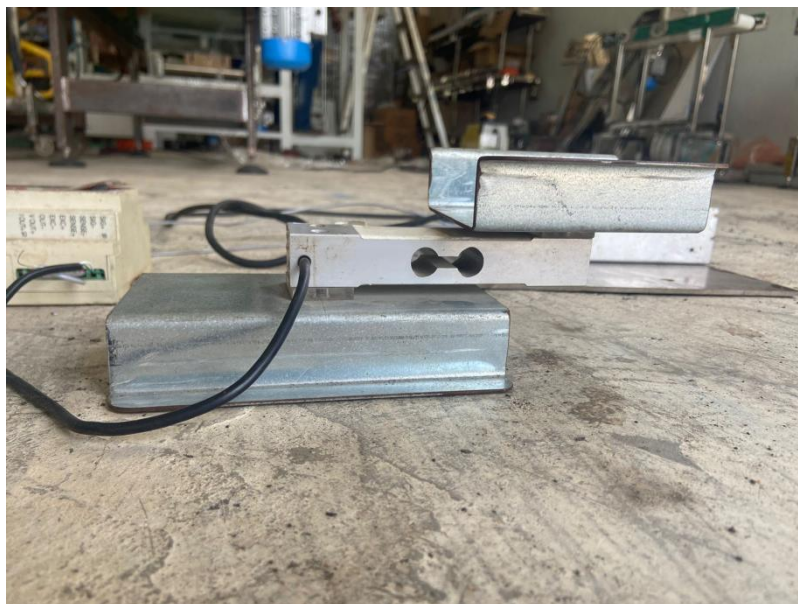
Fig 4.11 80KG load capacity load cell
