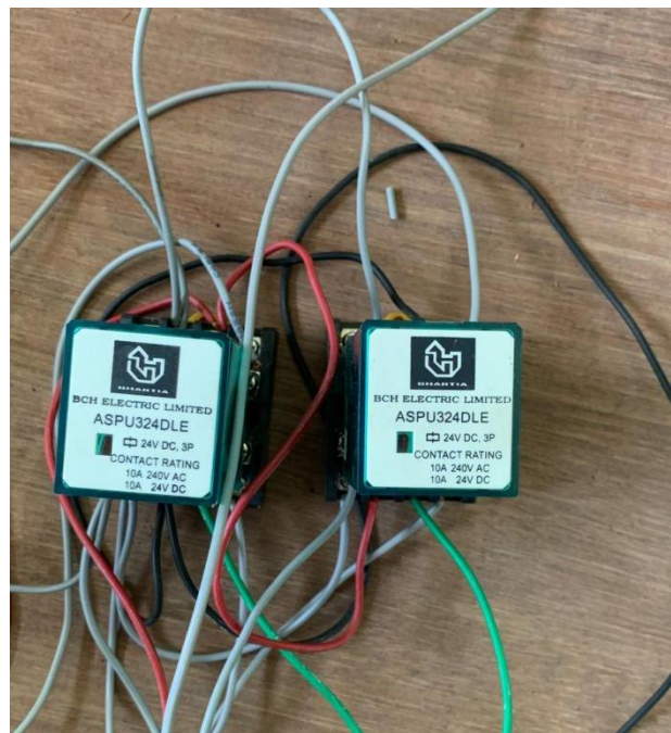
Fig 4.13 Relay used for Basic movements of AGV
