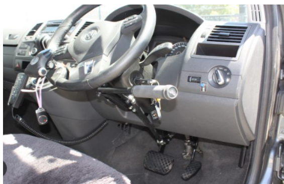
Fig: 2.1: Hand Control Twist And Pull Mechanism
