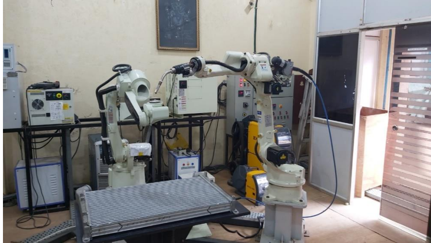
Fig: 1.7 : Fanuc Robots used for Laser Welding
