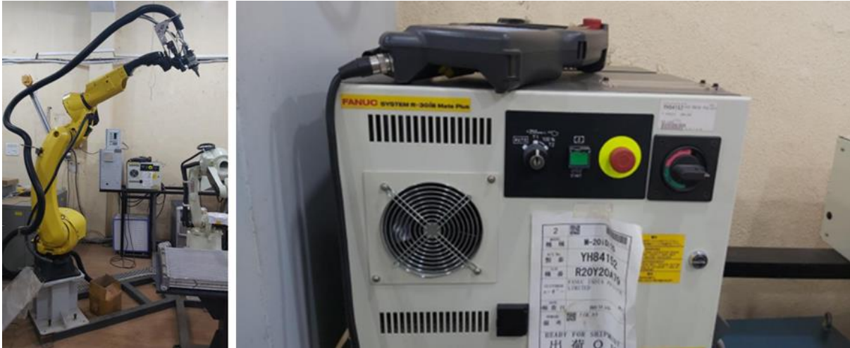
Fig: 4.3 : Fanuc Robot used for Laser Operation and the Teach Pendant Used to control the arm.
