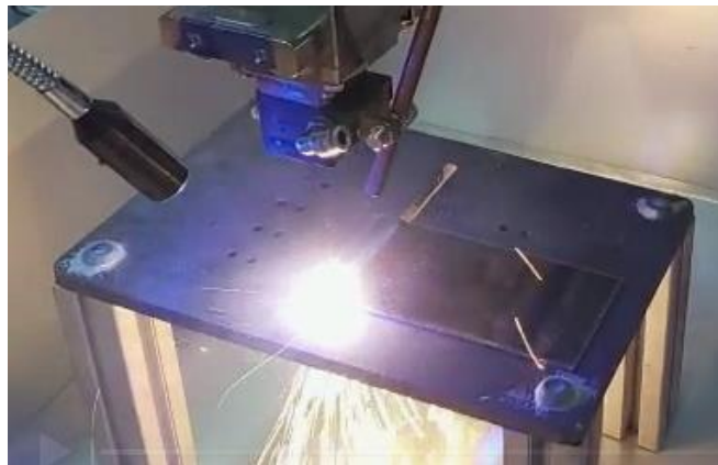
Fig: 1.5 : Laser Welding of Corten Steel
