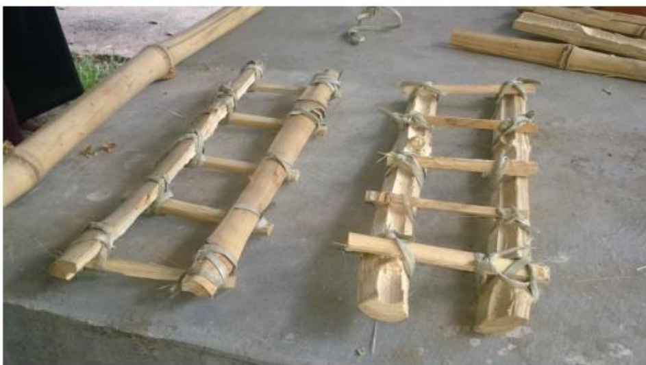
Tied bamboo reinforcements
