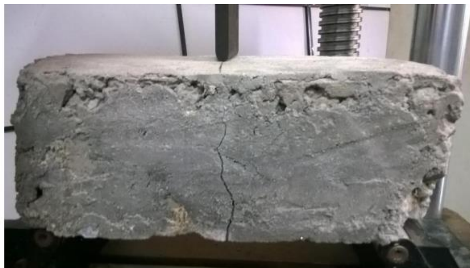
Crack in the beam due to bending
