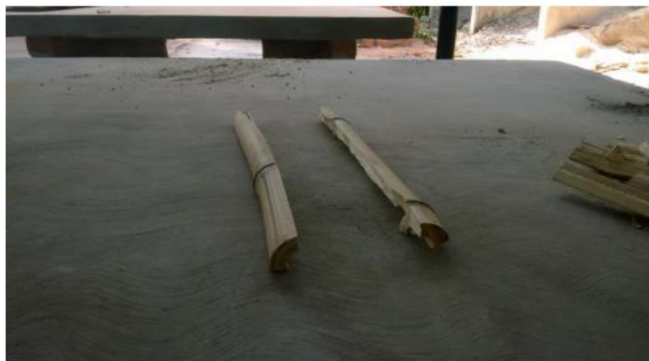
Splitting the bamboo culms
