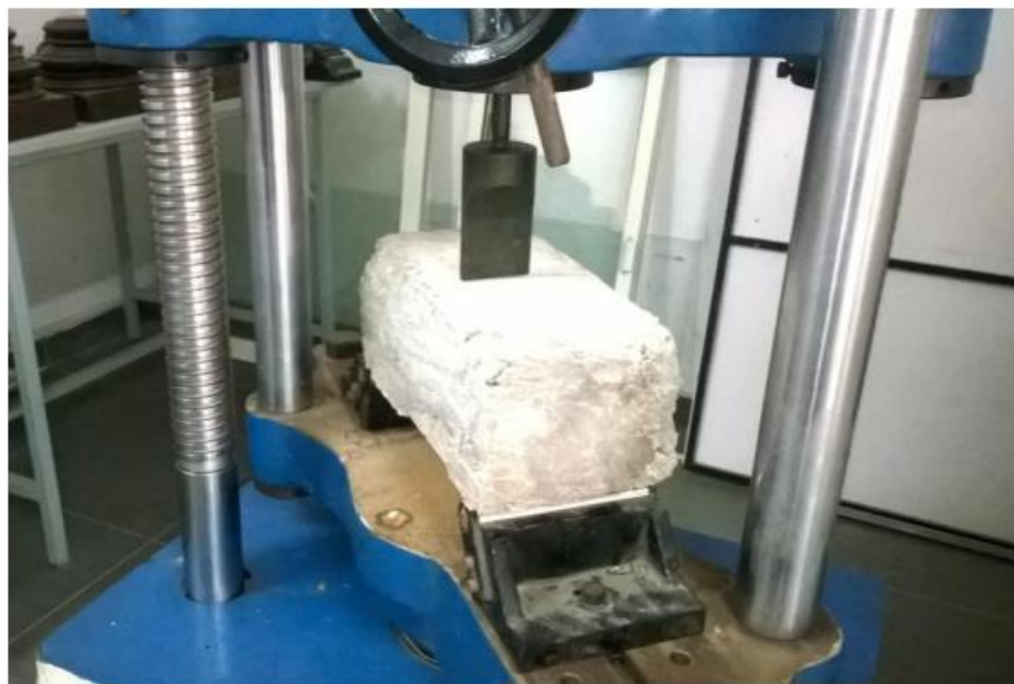
Beam placed in the loading unit of UTM
