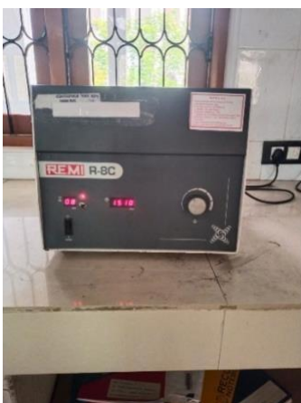
Fig 4.14. Centrifuge set for 4500rpm for 15 minutes
