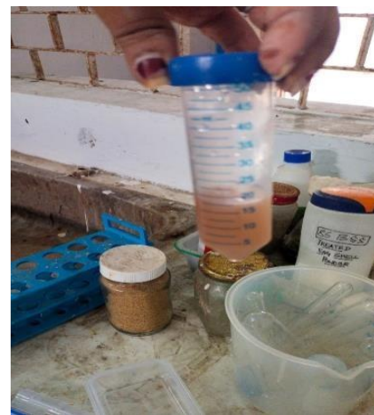
Fig 4.24. Extracted liquid in clean Tube for oil separation
