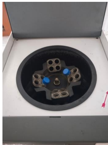
Fig 4.13. Tubes arranged in opposite manner inside the centrifuge machine
