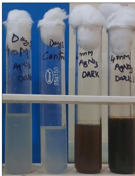
Fig: 5.5. Color change after the synthesis of silver nanoparticles
