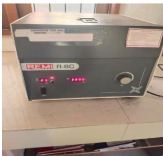
Centrifuge for 30 min in 4000 rpm
