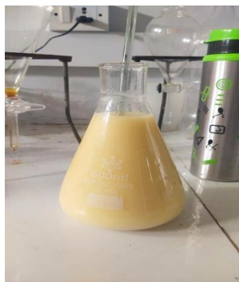
Added distilled water in biodiesel
