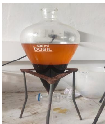
Glycerol and biodiesel were separated
