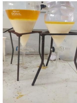
Biodiesel and impurities were separated
