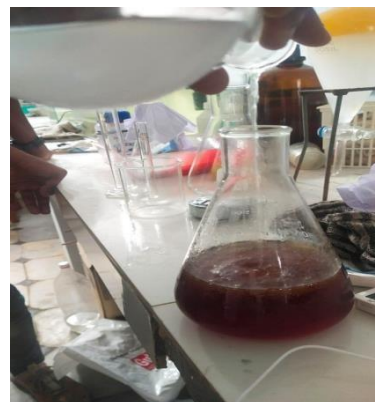
Add the Ethyl alcohol mixture in to Fish waste oil
