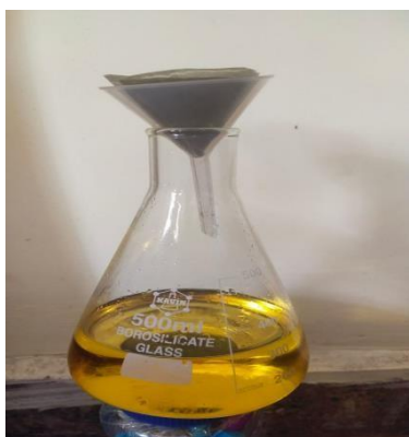
Filter the biodiesel by using filter paper
