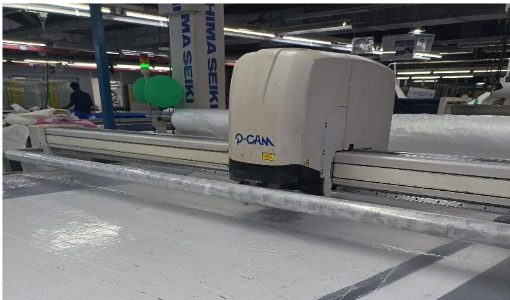
Figure 4.1(computer control knife)
