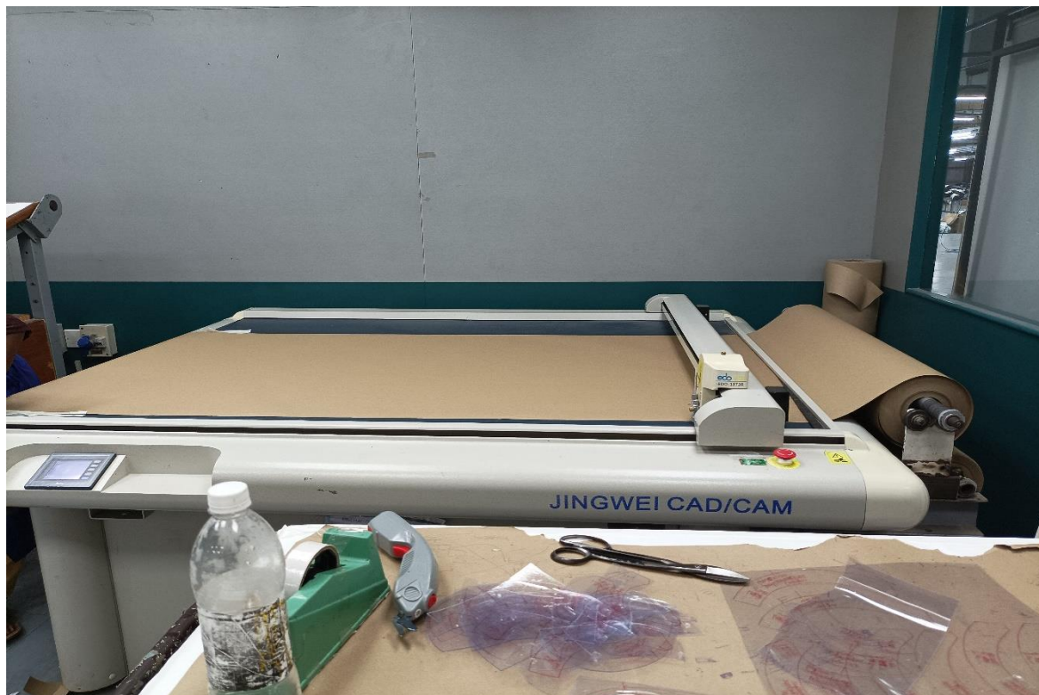
Figure4:(pattern CAD/CAM machine )
