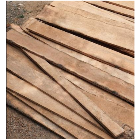
Coconut Tree Planks Are Used For Centering
