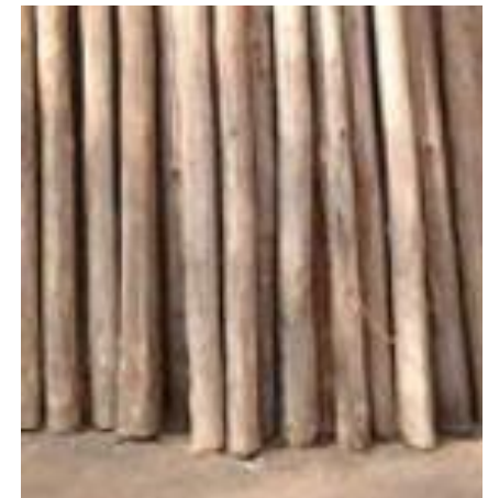
Casuarina Poles Are Used For Scaffolding And Supports
