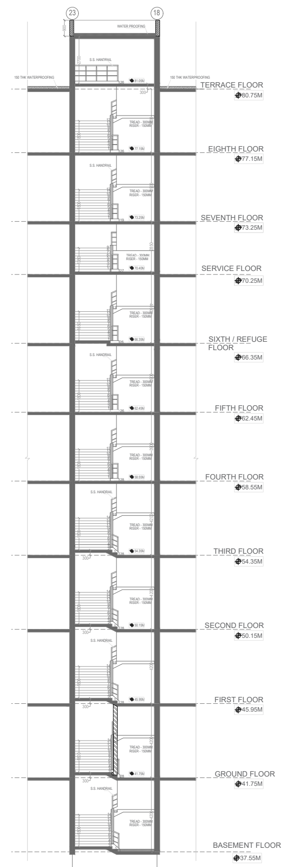
STAIRCASE 4 - SECTION BB
