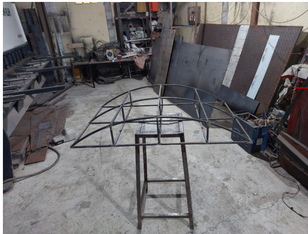
FABRICATION OF FORM WORK
