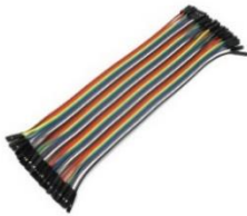
Fig-5 Jumper Wires
