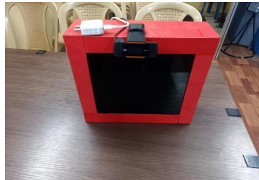
Fig. 8. Magic Mirror attached with Webcam
