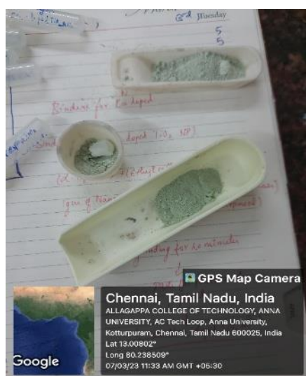
Fig.4.3:.. Prepared Copper Nitrogen co-doped TiO_2 photoanode
