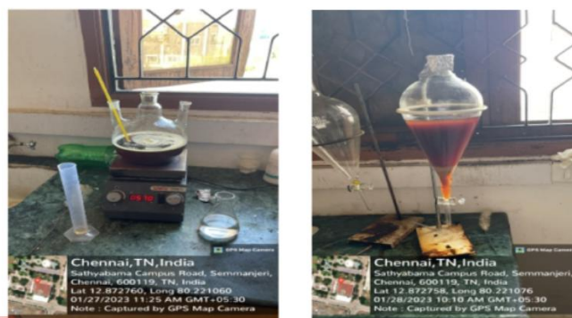
Fig. 4.2: a) Esterification of oil b) Separation of oil.
