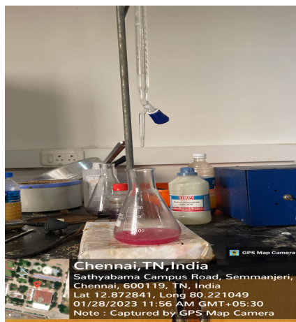
Fig. 4.8: Titration to find FFA%.
