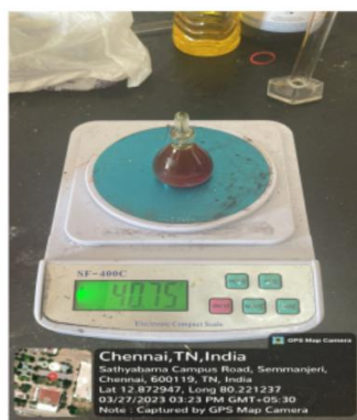
Fig. 4.6: Finding density using pycnometer.
