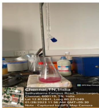
Fig. 4.8: Titration to find FFA%.
