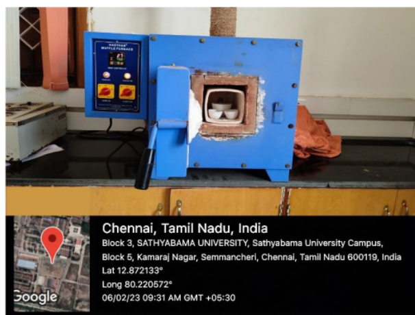
Fig. 4.2: Volatile Matter Determination
