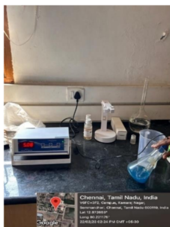
Fig 4.7: pH increment of copper acetate solution using pyridine
