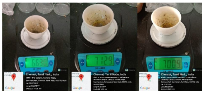
Fig 4.4 Estimation of moisture content
