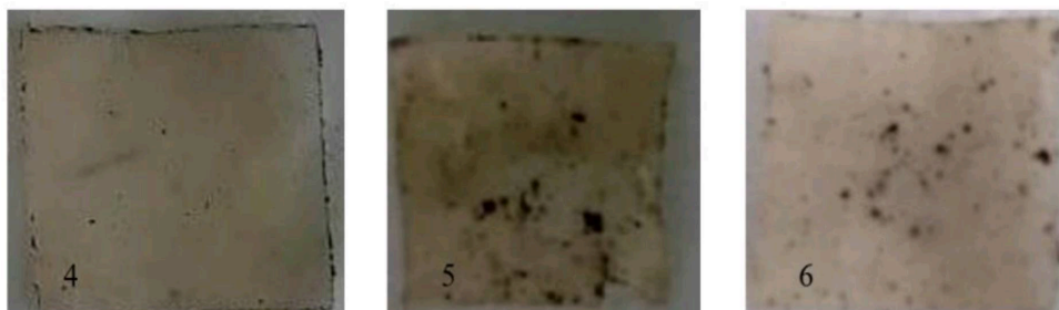
Fig.5.16; Soil burial Test. (1) Bioplastic on the day zero (2) size of bioplastic film was expanded on day two (3) More water and soil are entered into the bioplastic film on day four (4) Wide crack identified on bioplastic on day six (5) Some parts of bioplastic were diminished on day eight (6) most of the parts of bioplastics were completely degraded on day ten.
