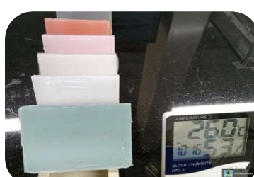
Fig 4.8 A set of samples was retained in room condition for 7, 14 and 21 days
