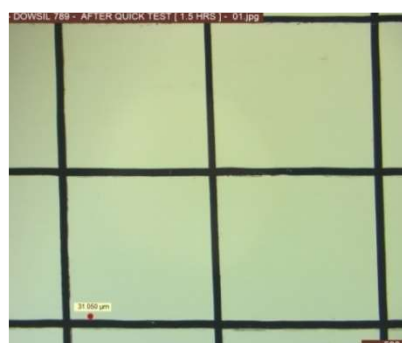
Fig 5.50 : After 1.5hrs [ Dowsil 789 @ 2mm ] – Place 01
