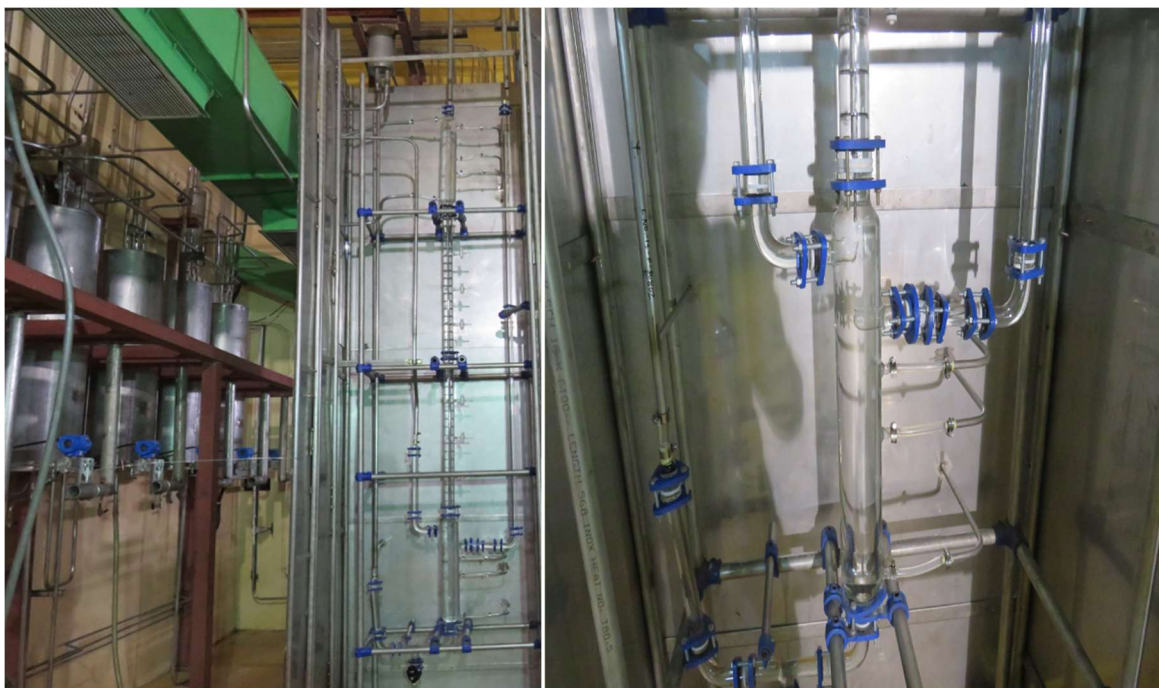
Fig: 4.4: Experimental pulse column and bottom disengagement section
