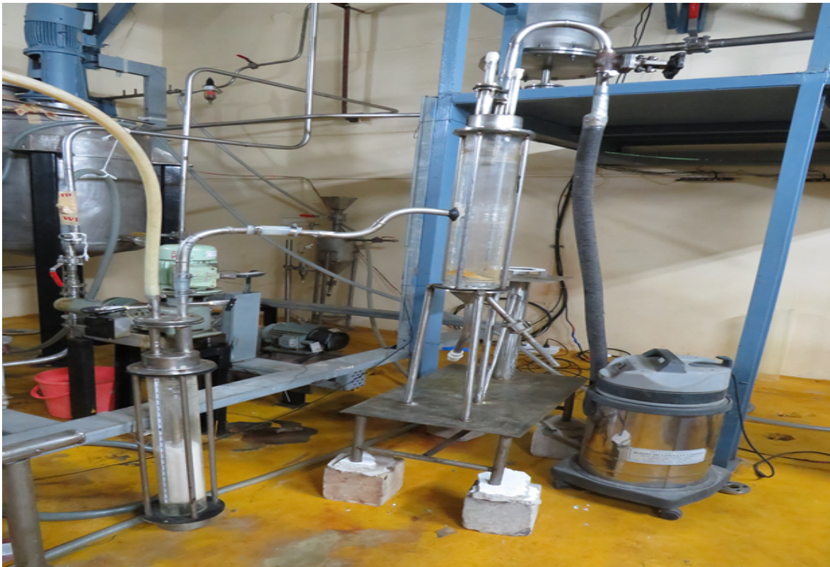
Fig 5.9: Actual experimental powder transfer set up (with fluidization) using the vacuum unit.
