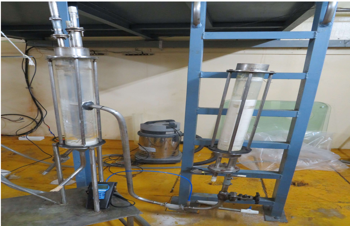
Fig 5.11: Actual experimental powder transfer set up (without fluidization) using Air Ejector.
