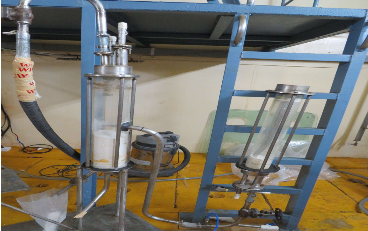
Fig 5.10: Actual experimental powder transfer set up (without fluidization) using vacuum unit.
