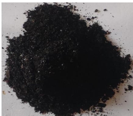
Fig.4.2 Preparation of Activated Carbon of MNP-PS
