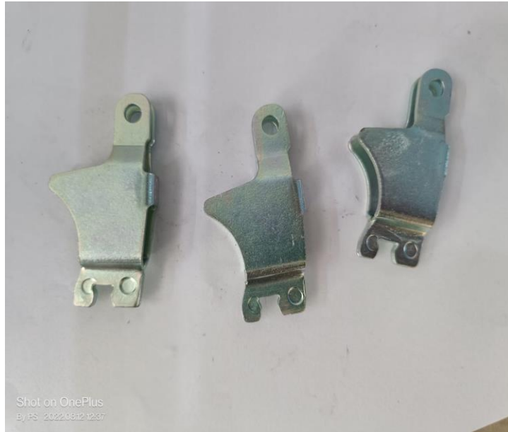
Fig 6.3 Final Finish for Strut
