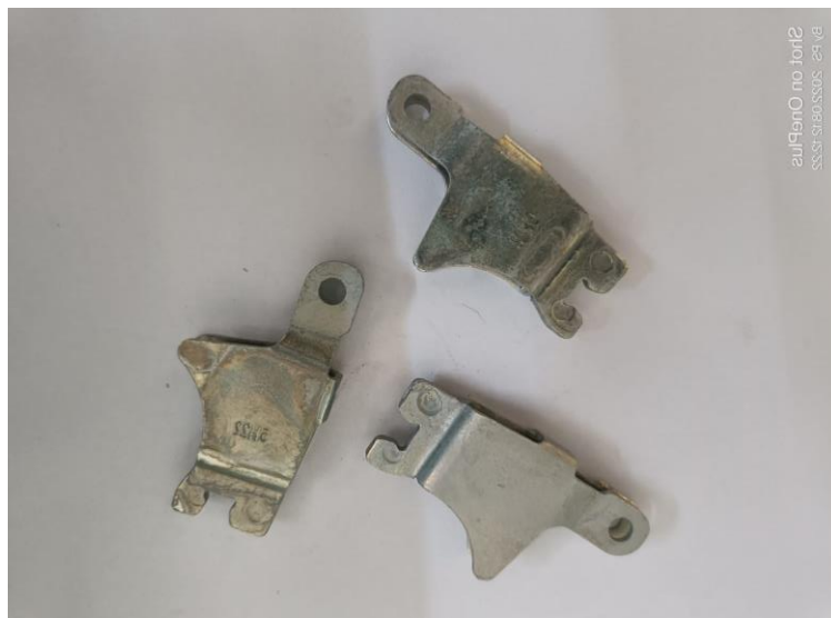
Fig 6.2 After Oven Finish for Strut
