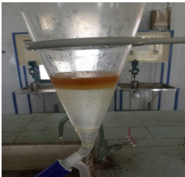
Fig 4.3 WASHING AND DRYING BIODIESEL
