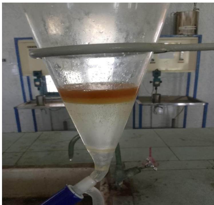
Fig 4.3 Washing and Drying Biodiesel
