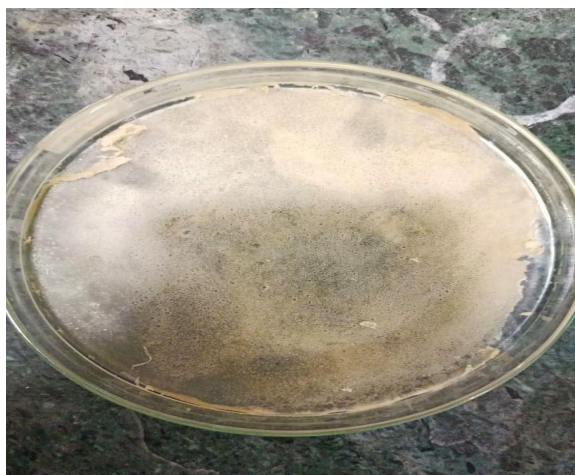
Fig.4.15: Sample B containing 1g of PEG,1g of Alginate,1g of Glycerol,1g of CMC and 1g of PVA.
