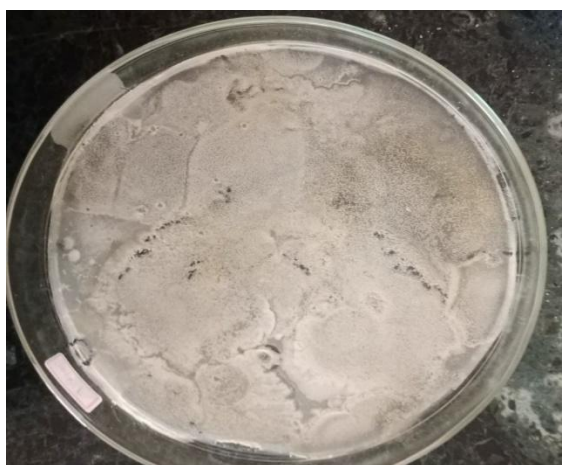
Fig.4.16: Sample C containing 2g of PEG,2g of Alginate, 2g of Glycerol,2g of CMC and 2g of PVA.
