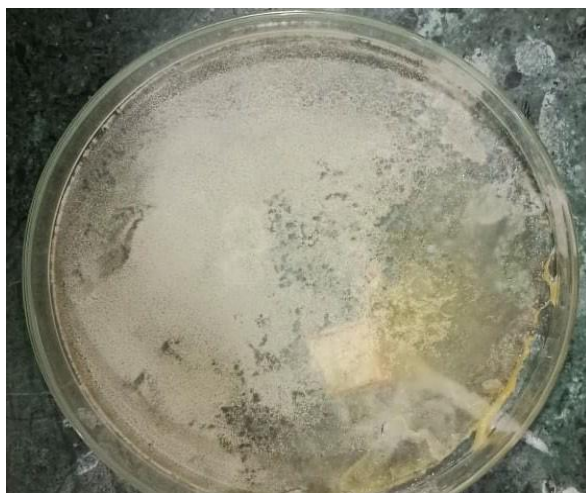
Fig.4.17: Sample D containing 2.5g of PEG,2.5g of Alginate,2.5g of Glycerol,2.5g of CMC and 2.5g of PVA.
