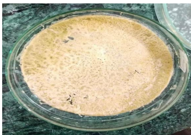
Fig.4.24: Sample K containing 2.5g of PEG, 2.5g of Alginate, 2.5 ml of Glycerol, and 2.5g of Starch.
