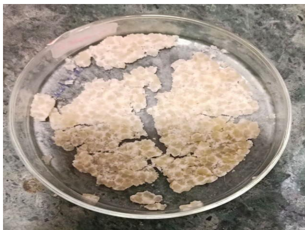
Fig.4.22: Sample I containing 2.5g of PEG, 2.5g of Alginate, 2.5 ml of Glycerol, and 2.5g of Starch.
