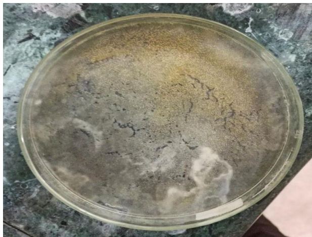
Fig.4.20: Sample G containing 1g of PEG, 1g of Alginate, 1 ml of Glycerol, and 1g of Starch.
