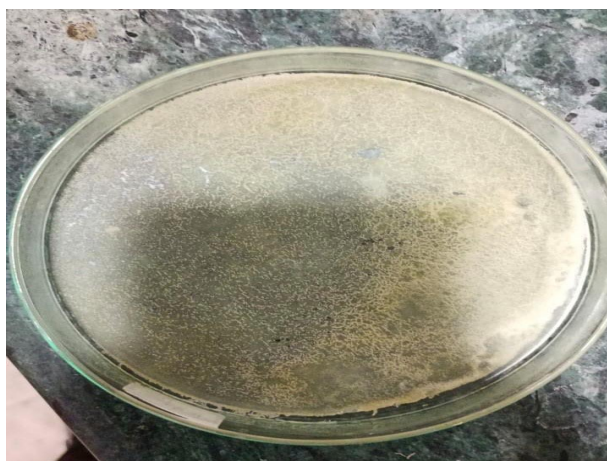
Fig.4.21: Sample H containing 2g of PEG, 2g of Alginate, 2 ml of Glycerol, and 2g of Starch.
