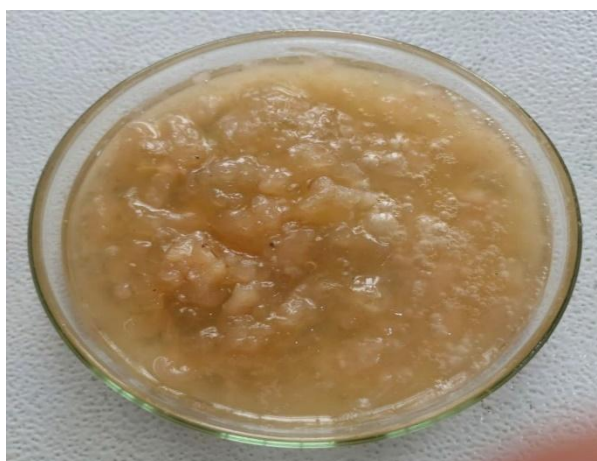
Fig.4.18: Sample E containing 4g of PEG,4g of Alginate,4g of Glycerol,4g of CMC and 4g of PVA.
