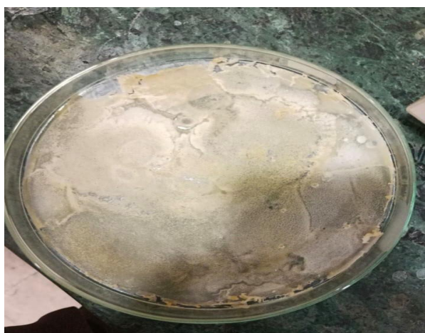
Fig.4.18: Sample E containing 4g of PEG,4g of Alginate,4g of Glycerol,4g of CMC and 4g of PVA.
