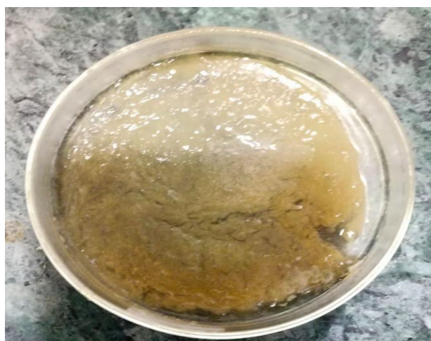
Fig.4.25: Sample L containing 1g of PEG, 1g of Alginate, 1 ml of Glycerol, 1g of Starch, 1 ml of PVA.
