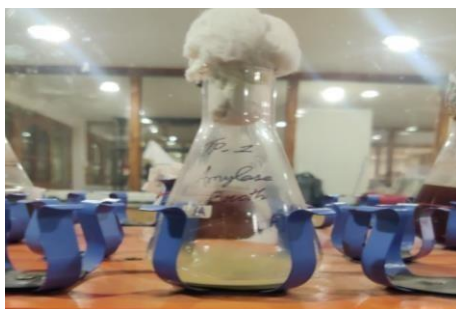
Fig 5.4 Production of amylase enzyme by shake flask method
