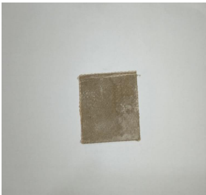
Fig 4.7:- Testing sample of Geopolymer panel
