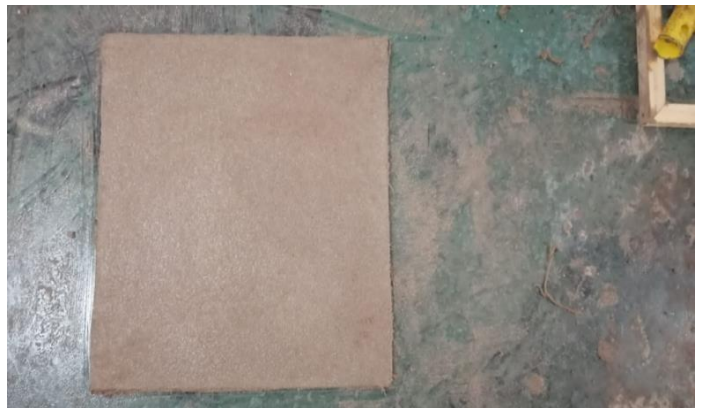
Fig 4.2:- fabricated Geopolymer panel
