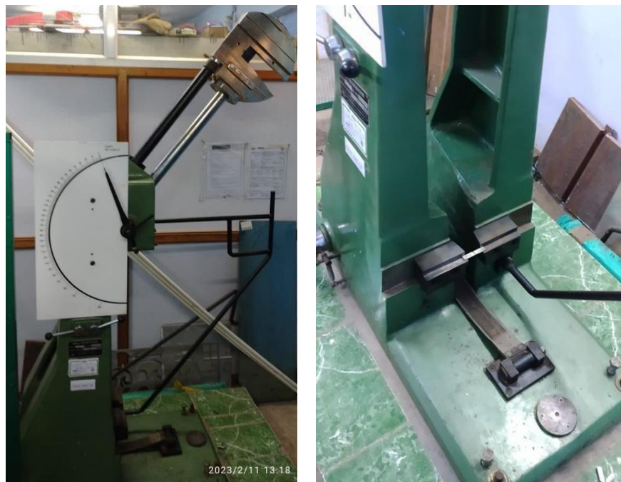
Fig. 4.13: Charpy impact test setup
