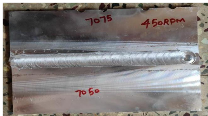
FIGURE 4.3 FSW of AA7075 and AA7050 at 450 rpm
