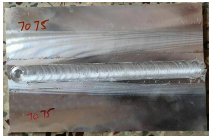
FIGURE 4.5 FSW of AA7075 at 450rpm
