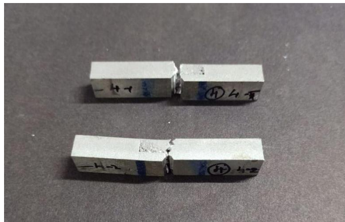
FIGURE 5.13 Impact test specimens after testing
