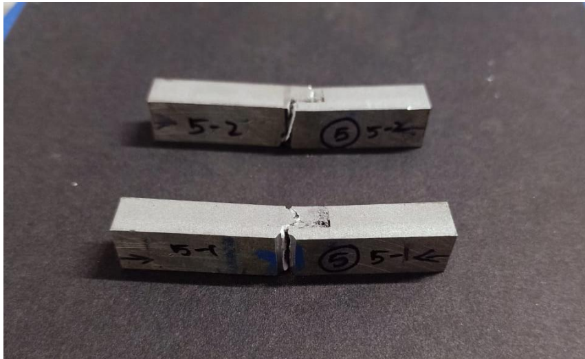
FIGURE 5.2 Impact test specimens of FSW on base material plates
