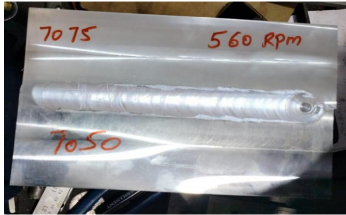
FIGURE 4.4 FSW of AA7075 and AA7050 at 560rpm
