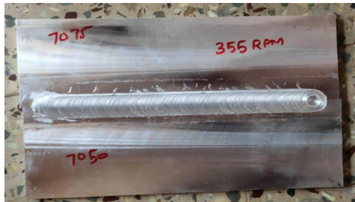
FIGURE 4.2 FSW of AA7075 and AA7050 at 355rpm
