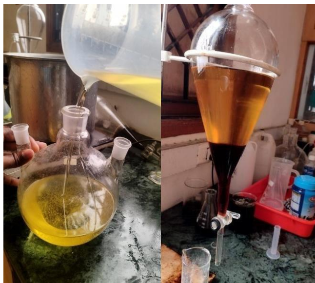
Fig 4.5: Transesterification of Biodiesel
