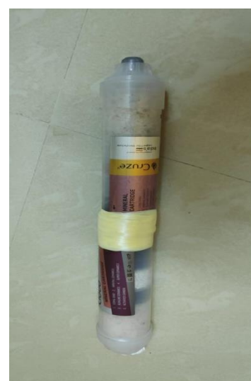
Fig 5.6.rGO powder infused pre-filter
