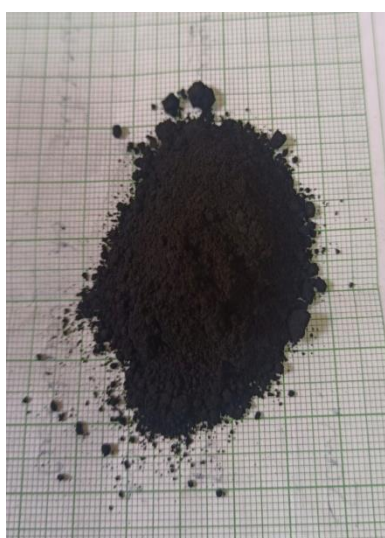
Fig 5.5. Synthesised rGO powder
