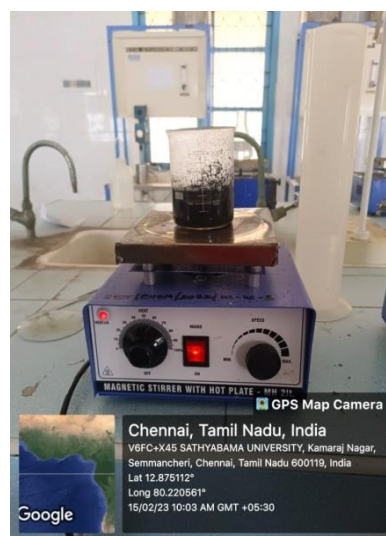
Fig 5.3. Magnetic stirred for 30 min at a low temperature of 80 °C
