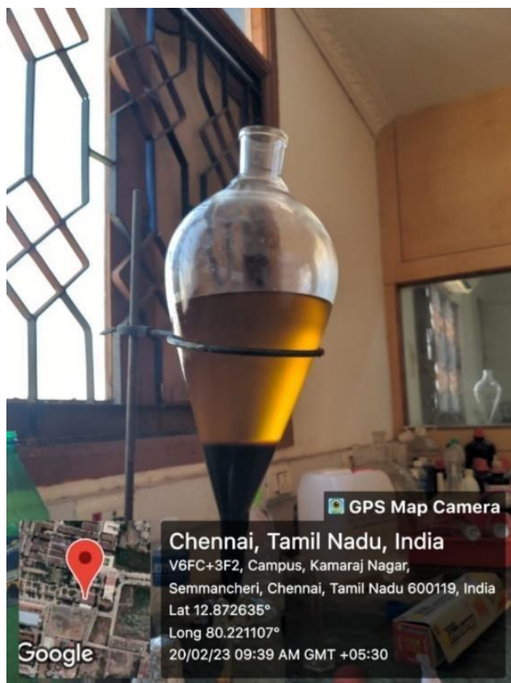
Fig 4.6 Tranesterification of karanja Oil
