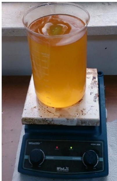
Fig.4. 2. Mixing process of safflower oil and methyl alcohol
