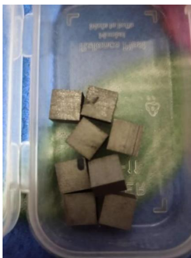
Fig4.1 . sample pieces obtained from EDM wire cut process
