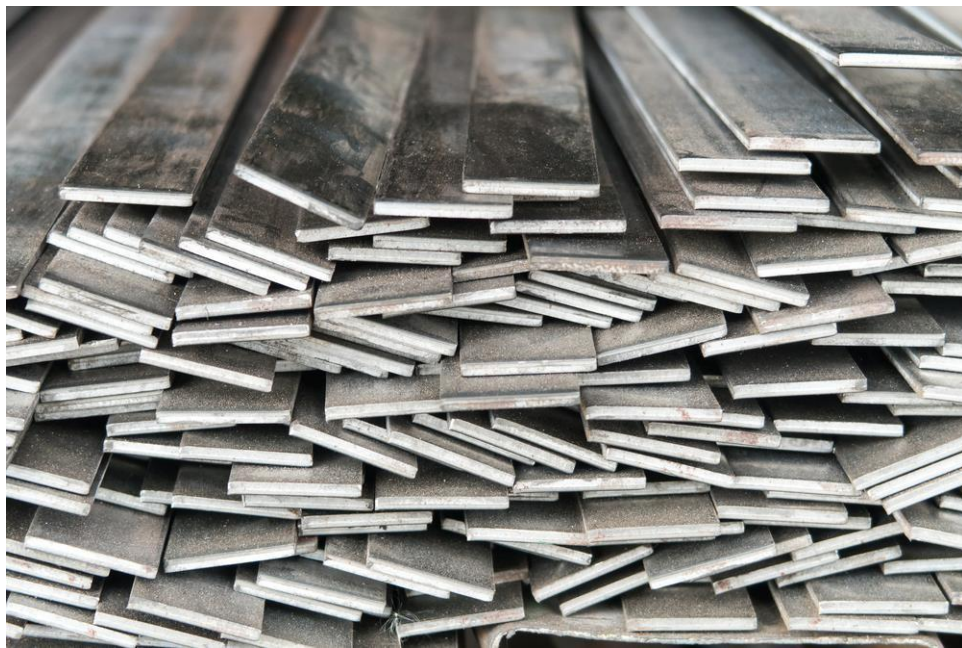
Fig: 4.2 : 1-inch 5mm steel flat
