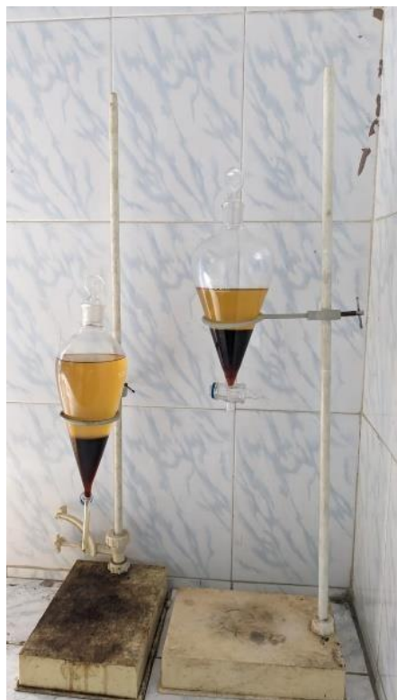
Fig: 4.2 Separation of Glycerin with Oil
