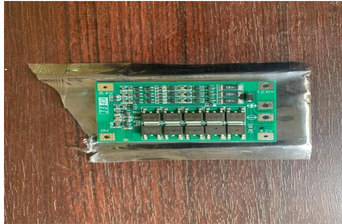
Fig 1.3: Battery Management system.
