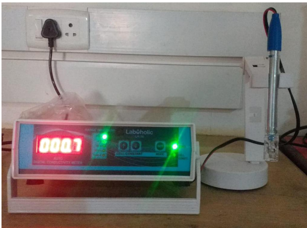
FIG 4.18: ELECTRICAL CONDUCTIVITY METER
