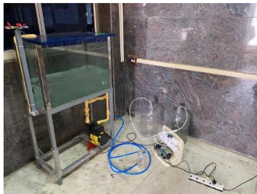
FIG 4.10: NANO BUBBLE GENERATOR WITH RO UNIT
