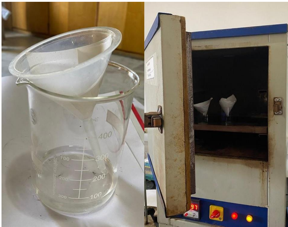
FIG 4.13: TSS FILTER WITH HOT AIR OWEN
