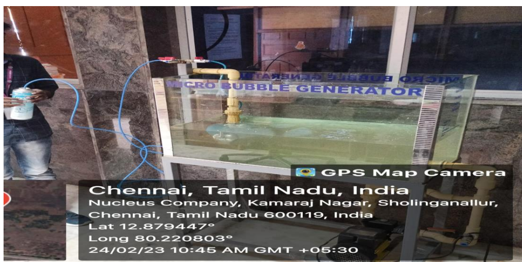
Fig. 5.4: Generation of oxygen nanobubbles using micro-nanobubble generator
