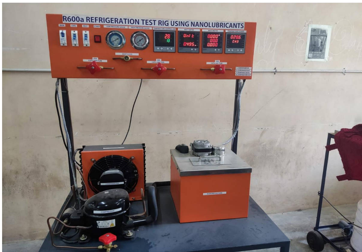
Figure 4.1: R600a experimental test rig
