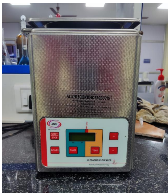
Figure 4.4: Nano lubricants undergoing sonification process
