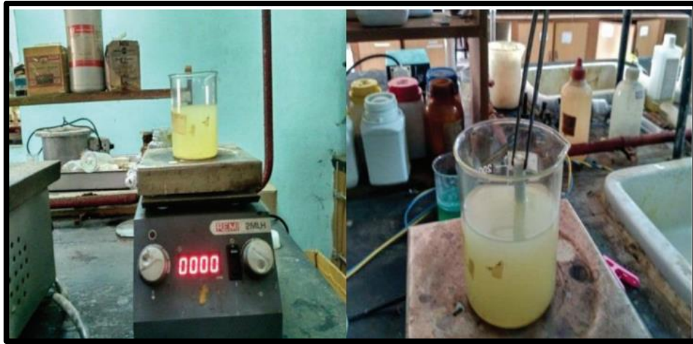
Figure 1.2: Prepared Nanofluid using Magnetic Stirring Method
