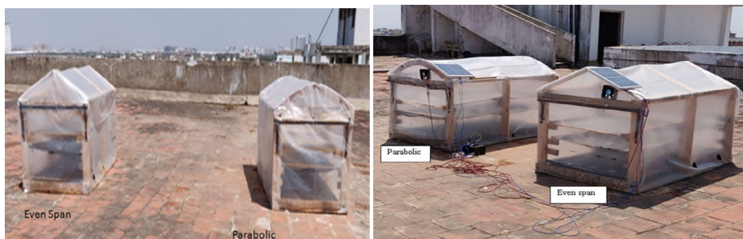
Figure 2.10: Experimental setup of span and parabolic Drying GHSD
