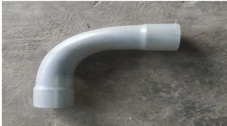
Figure 4.3: PVC Pipe (Chimney)
