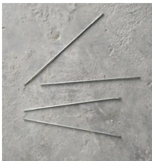
75mm steel rod (Ribs)
