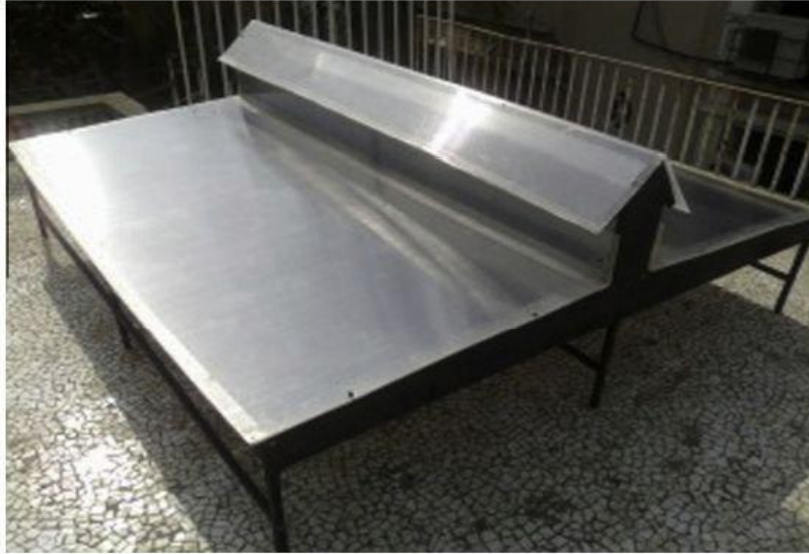
Figure 2.9: Solar conduction dryer[8]
