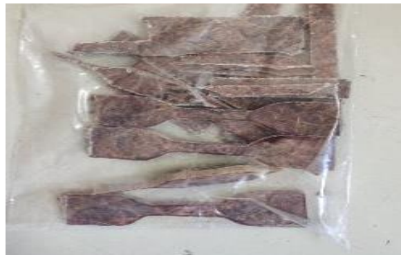
Fig:4.16: Tensile, flexural and impact samples of treated banyan root fiber composite
