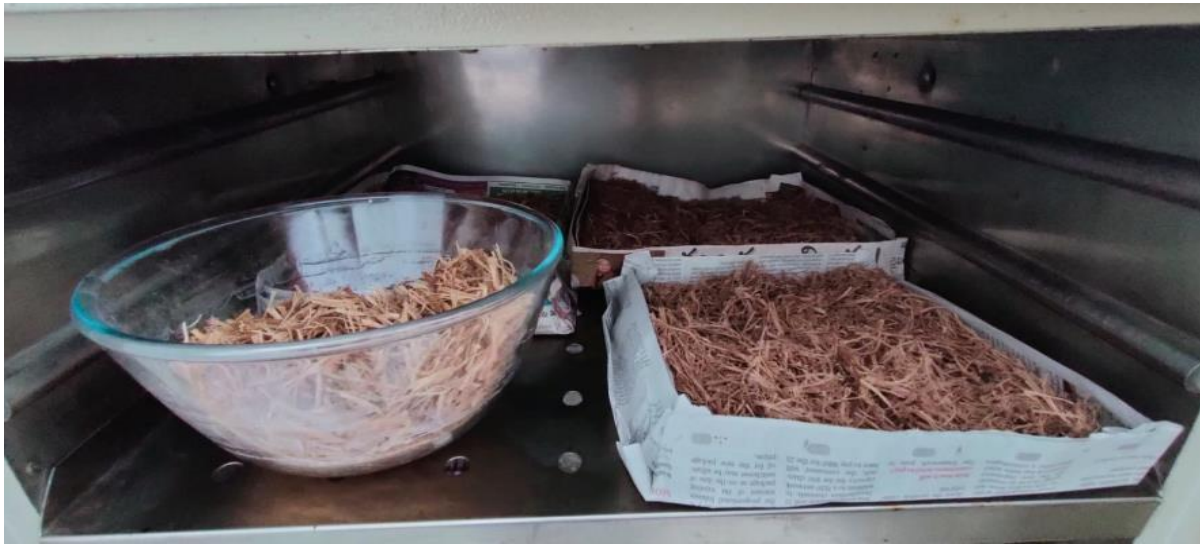
Fig:4.9: Removing the moisture present in the fiber using oven
