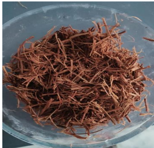
Fig:4.6: Fiber treated with 10 % Ca(OH)_2 chemical
