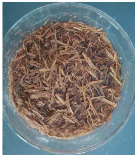
Fig:4.4: Fiber treated with 5 % \text{Ca}(\text{OH})_2 chemical
