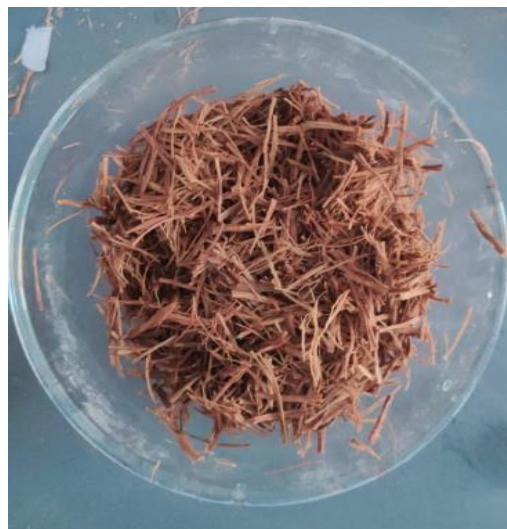
Fig:4.8: Fiber treated with 15% \text{Ca}(\text{OH})_2 chemical
