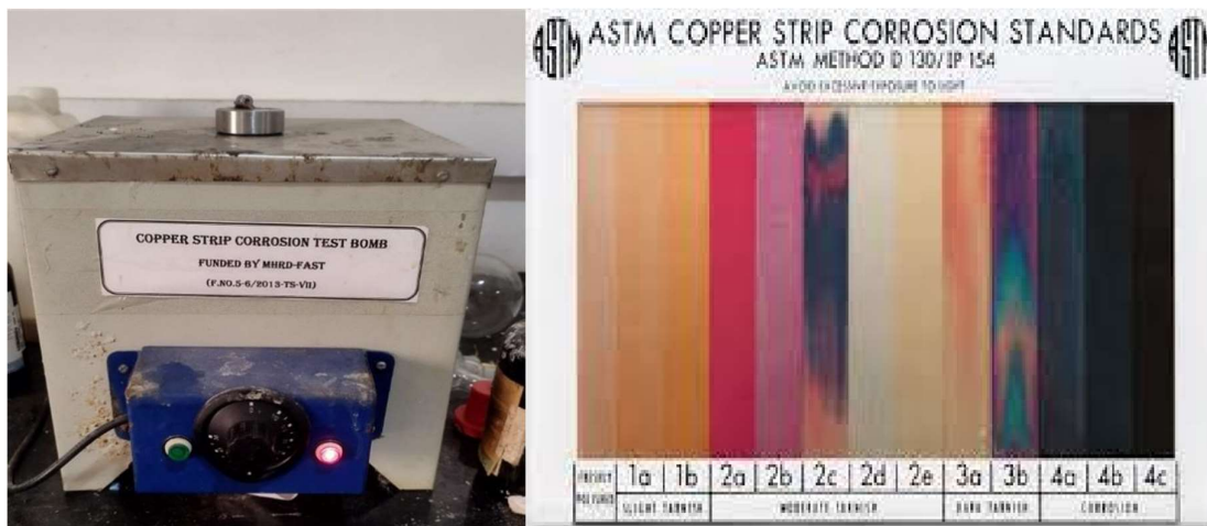
Fig 4.14 Copper strip corrosion test @60°C for 3 hrs
